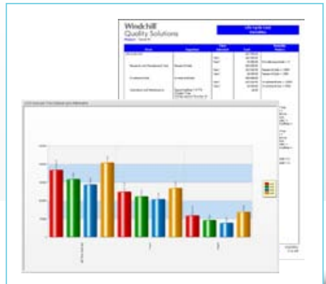
Windchill LCC computes overall system costs as well as line-item costs.
